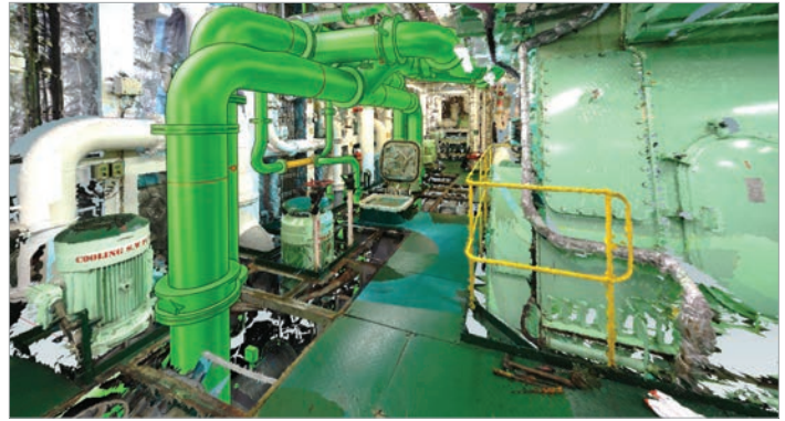
Laser data integrated with the 3D model
